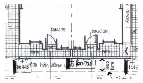
Once the retaining wall has been constructed the original footway would be reduced from a width of approximately 1.8m to 1.35m. The photograph above shows a footway of less than 1.35m but this will be increased by filling between the new retaining wall and the footway. An extract from the proposed plan copied above indicates that once the works are completed the footway would be 1.35m wide.
